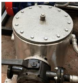
Bitumen (Asphalt) Filter
